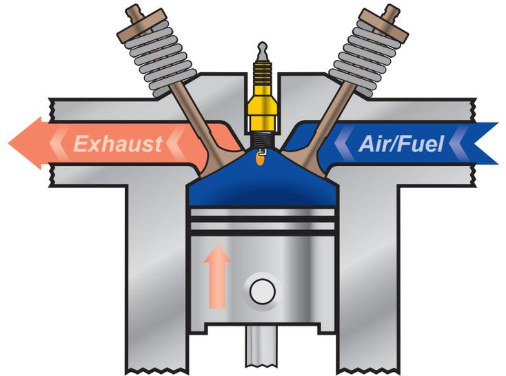
Spark occurs at the end of the stroke when the piston is "Top Dead Center", this is when the piston is at the highest point of its apex.
